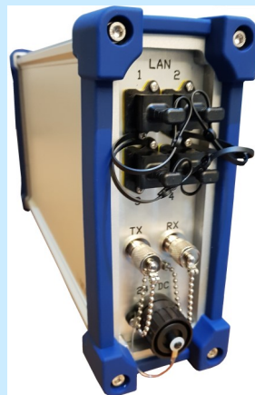
Rear of outdoor modem showing weatherproof connectors (4 x Ethernet, Tx, Rx and DC input). A mounting bracket allows the modem to be secured in place. Several mounting options are available and can be customised to suit individual requirements.
